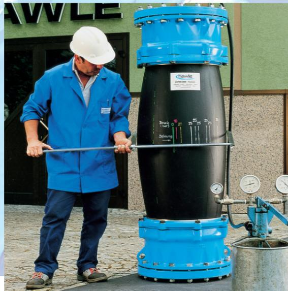
Pressure test: **SYSTEM 2000 Flange Adaptor** DN 400 with PE pipe o. d. 450 mm (wall thickness 28,4 mm) at 23 bar
